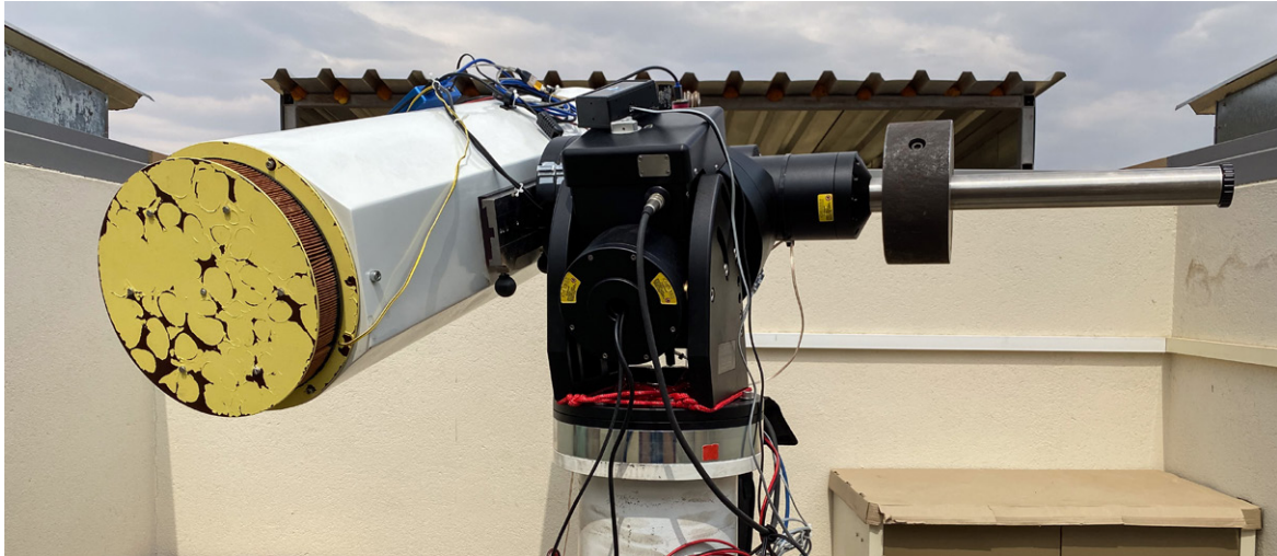
Abb. 1: IAS 10" Newton Remote Telescope 2
